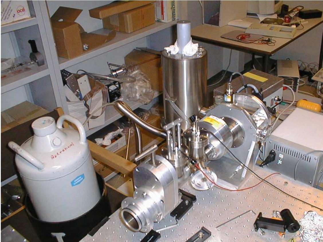
**Figure 3.6** The beam-line interface, holding a light source and a Fe-55 source among other things; and the CCD camera, including read out electronics.
