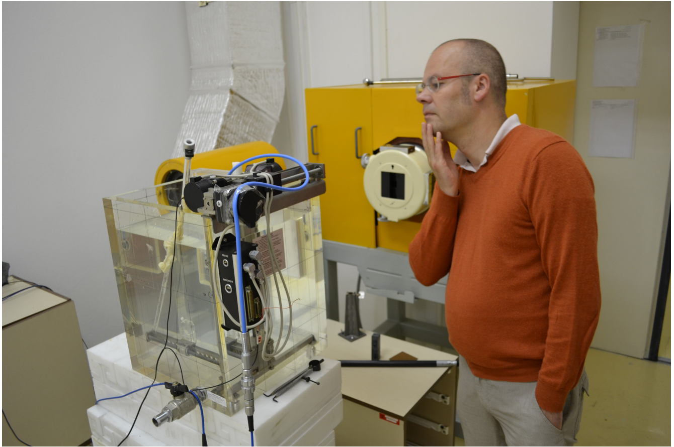
The yellow box holds the Co-60 source, behind the tank an additional collimator is visible which can be mounted in front of the Co-60 unit.
