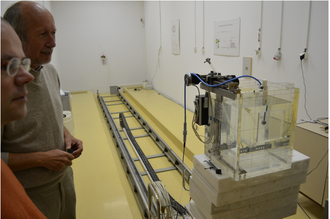
In the Co-60 irradiation room. Water tank is here holding a Markus ionization chamber. The dose-rate can be reduced by increasing the distance to the Co-60 irradiation unit.
