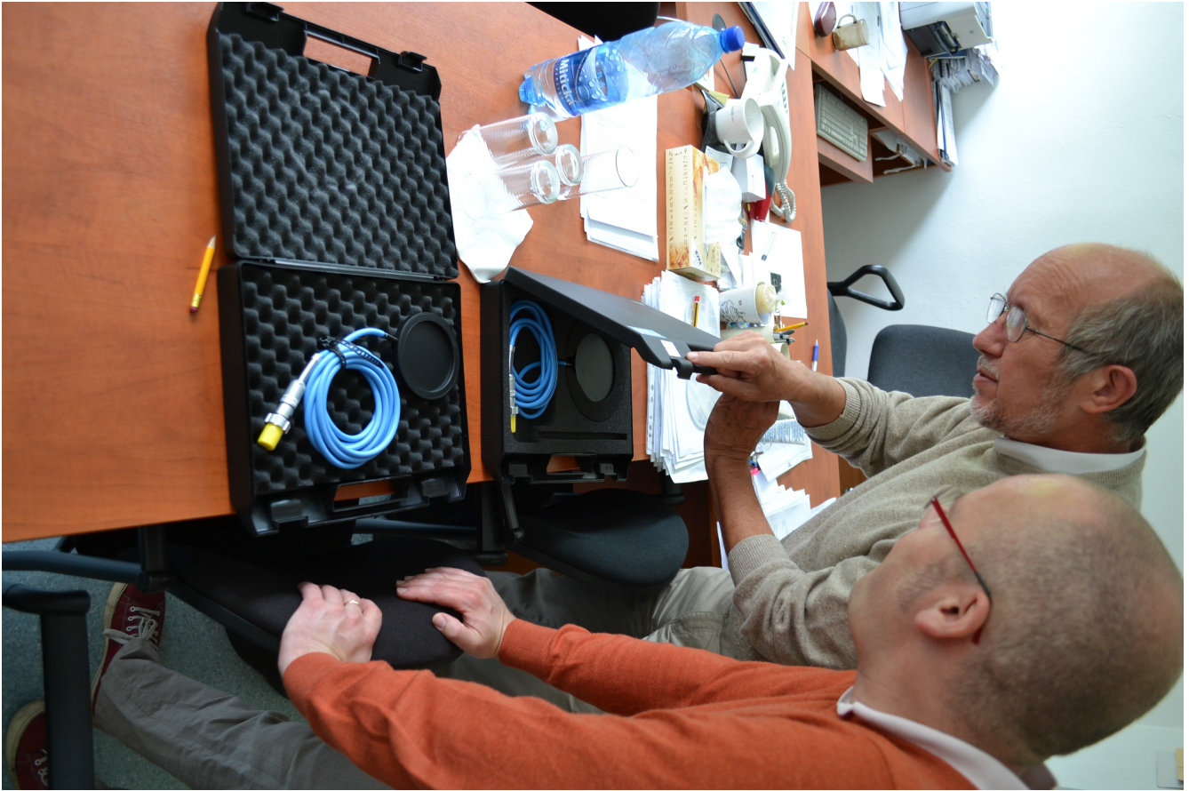
Roos ionization chambers from PTW, well suited for measuring depth-dose curves of pencil shaped ion beams.
