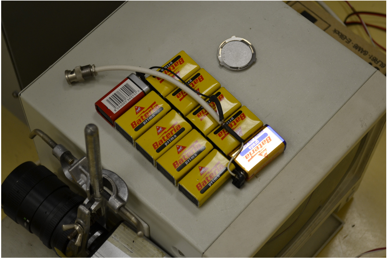
How to make 90 Volts... :)
